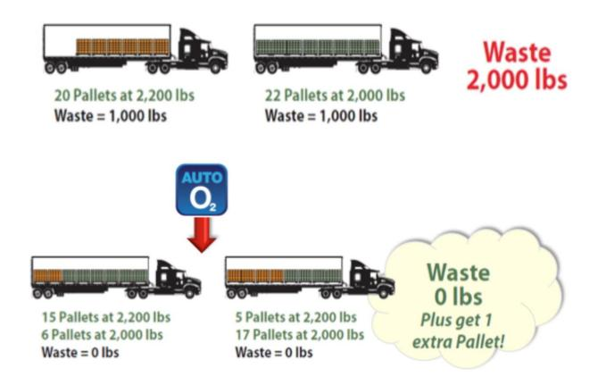
Auto $O_2$  uses a variety of information including time-phased demand, product dimensions and weight, as well as how it is palletized, and it's "stack ability" to determine how to best use the valuable lane-specific truck capacity. Auto $O_2$  cautiously uses requirements from subsequent days to ensure that the load is truly full. In the real world, loads are 4-8% bigger, meaning that over the course of time, 4-8% of all shipments can be eliminated.
